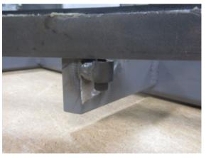
Screws to attach Rear Quarter Frame to Frame Fixture Exterior Impact Side
