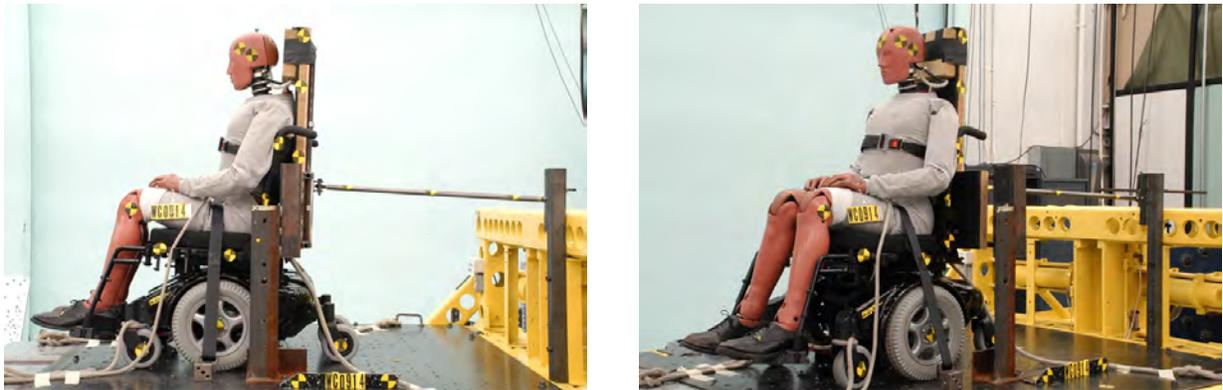
Figure 2.60 - Pre-test photos for the second rear-impact sled test of a BME student-designed vehicle-mounted head-and-back restraint
