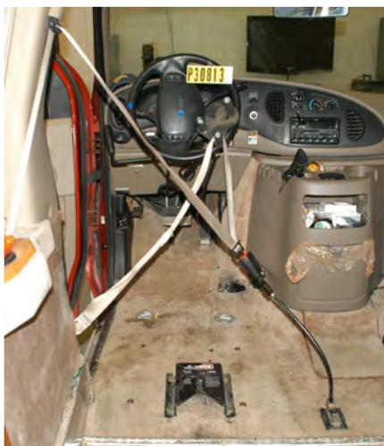
OEM seat belt used in the passive mode
