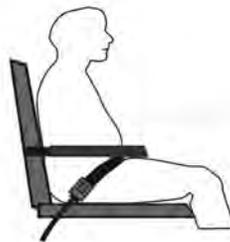
Proper positioning of a vehicle-anchored lap belt low on the pelvis with wheelchair arm supports that attached to the wheelchair back-support posts
