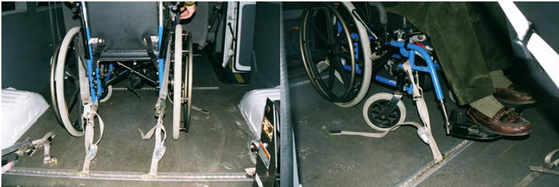
**Damaged Wheelchair With Right Arm Support Bent Outward and Postural Belt Torn from Wheelchair Anchor Point**
