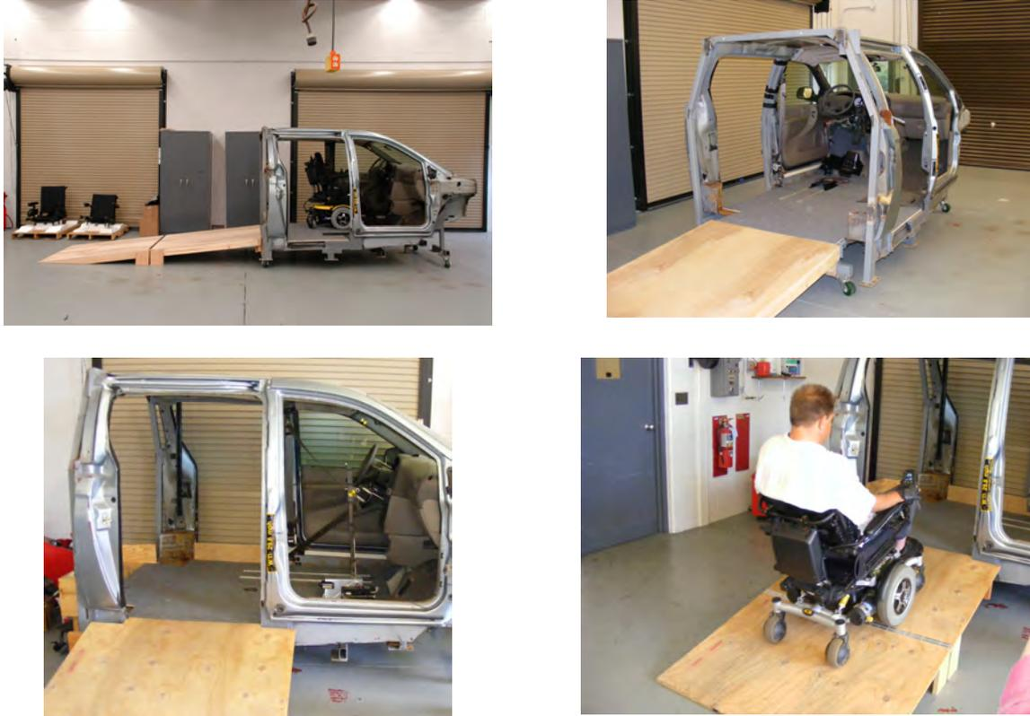
Figure 2.14 -Minivan buck in UMTRI high-bay laboratory with rear-entry and side-entry ramps used for wheelchair driver ingress and egress to evaluate prototype restraint-system designs
