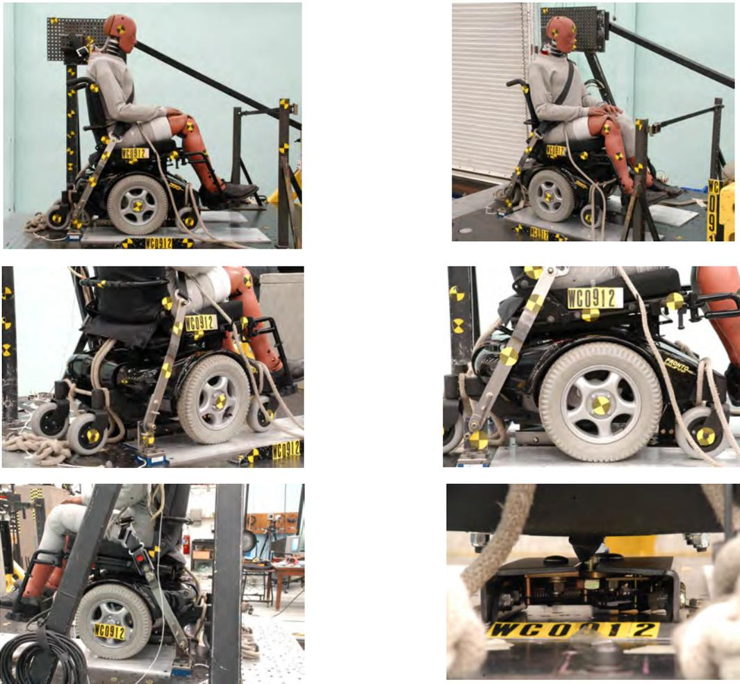
Figure 2.26 -Photos of the prototype pivoting-bar lap/shoulder belt restraint system prior to conducting the third and final 48-kph, 20-g frontal sled-impact test
