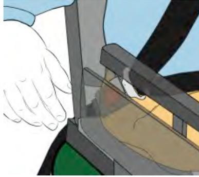
Lap belt threaded into opening between the wheelchair seat and back support to achieve proper positioning low on the pelvis
