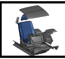
All simulations were run in the front passenger seat environment of a 2014 Honda Accord model (pictured left). A pre-crash simulation with **In-Crash HBM**
