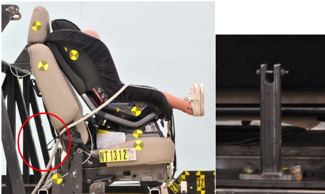
Figure 7. Side view of the “low” tether anchorage location representing a seatback-mounted tether, plus a rear-view close-up of the hardware.
