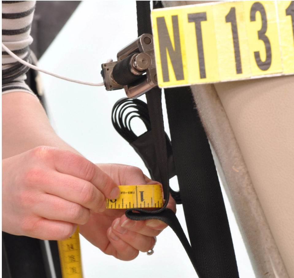
Figure 9. Measuring slack in tether post-test.
