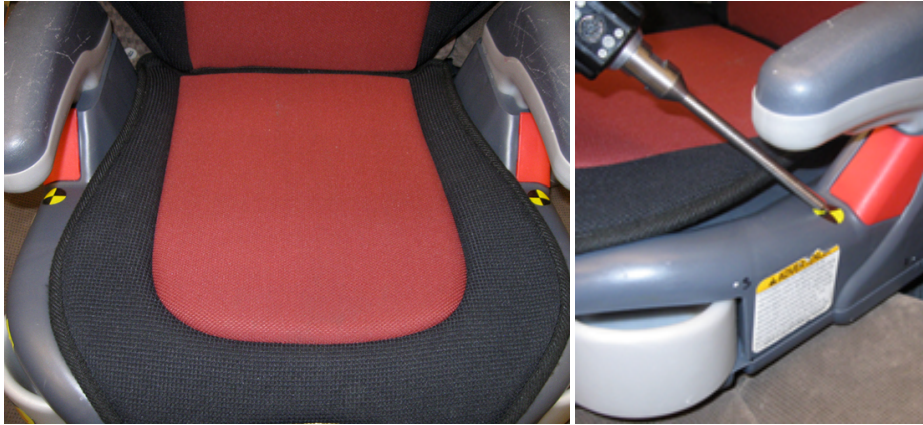
Figure 17. Example bilaterally symmetrical points on booster seat
