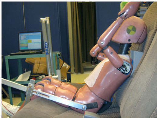
Figure 33. Propping ATD head off the seat back
