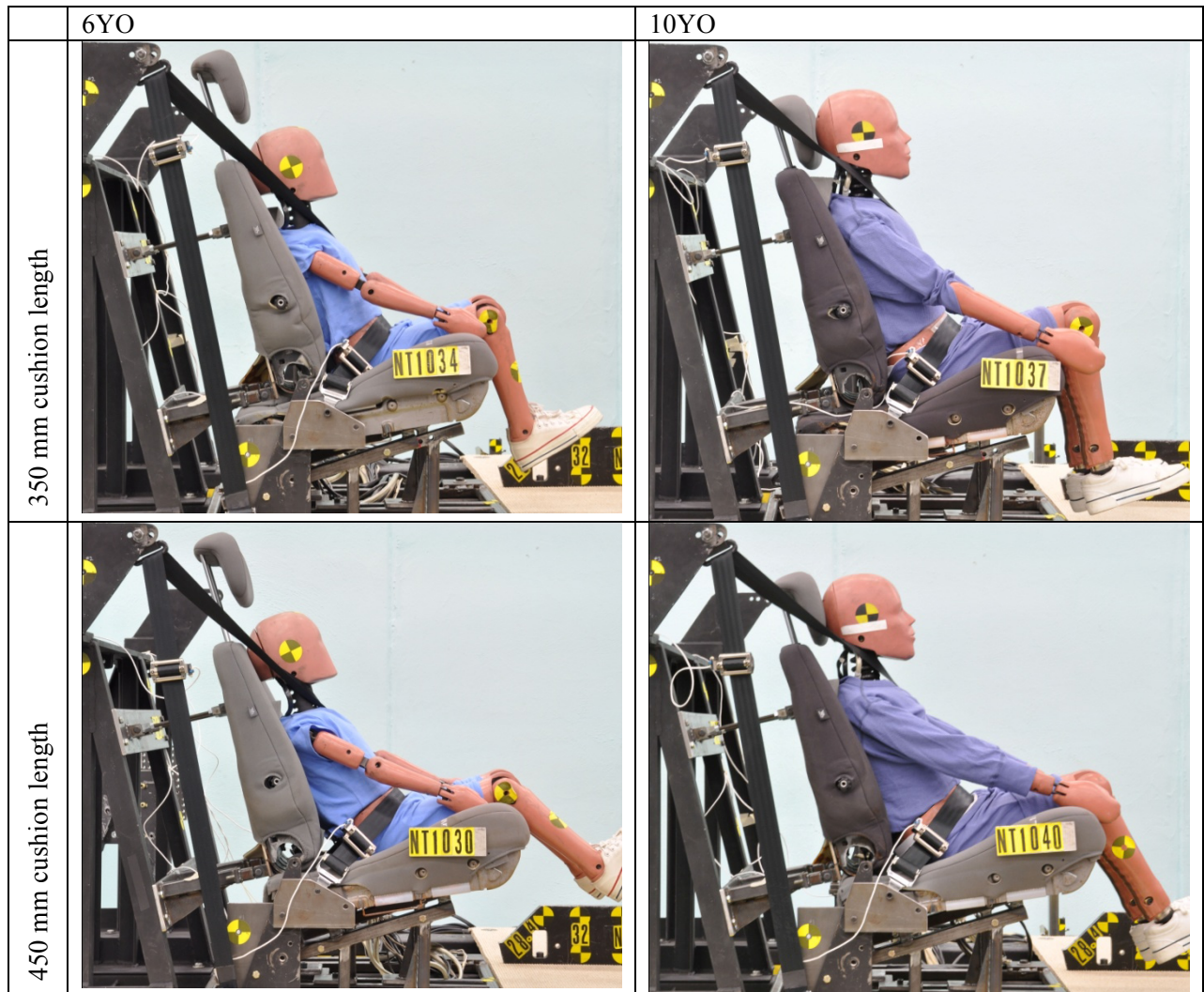
Figure 7. Initial positions of 6YO and 10YO ATDs in vehicle seats with cushion lengths of 350 and 450 mm
