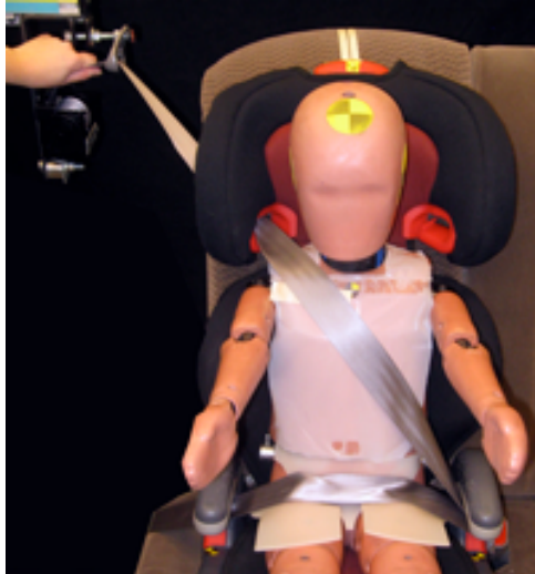
Figure 41. Feeding the shoulder belt into the retractor
